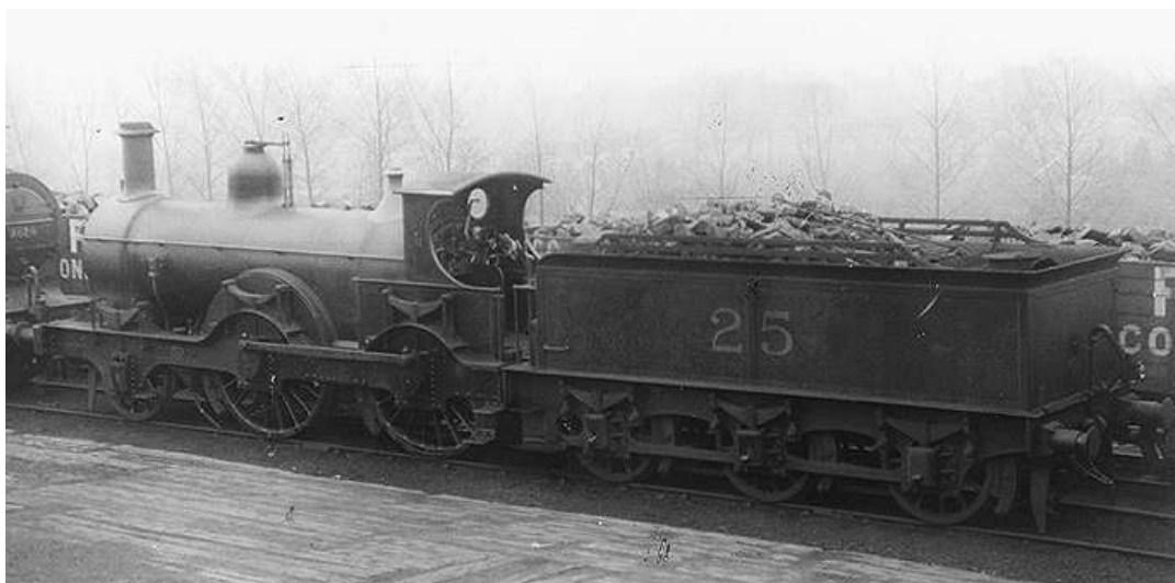
Fig 2: Midland Railways' locomotive no. 825, one of the same class of locomotives as that involved in the Kildwick crash. No. 819 was pulling the mail train; no. 814 was used by Capt. Tyler in his stopping-distance tests.
